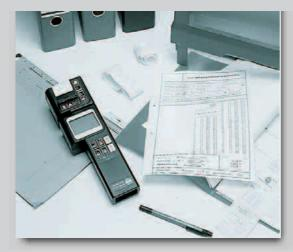
The tedious calculations required by the ventilation standards (error calculation, uncertainty of profile/location etc.) are made at a later time in the office. Assignment of the measured data to the location, including date and time as well as additional parameters (temperature, pressure, humidity), is absolutely necessary. At worst, it may turn out afterward that the measurement has to be repeated due to the large measurement uncertainty.
