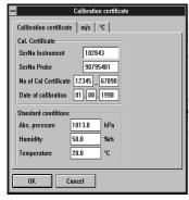
The deviations indicated in the calibration certificate can also be included when logging the results of the measurement in the PC. This leads to significantly better measurement results and fewer uncertainties.
