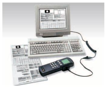
The measured data saved in testo 400 are transmitted to your PC at the touch of a button. Tedious written work is no longer necessary. The results of the measurement are printed in a standard form (see next page, step 6).
