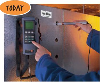
The testo 400 is simply attached via a magnetic holder to the ventilation duct. The engineer then always has one hand free. The data relating to the location such as location name, coordinates, duct area, correction factor etc. are automatically read into the measuring instrument via the barcode. The coordinates required for the grid measurement are shown in the instrument display (see page 1). The depth specification on the vane telescope hugely reduces the work in the field.
